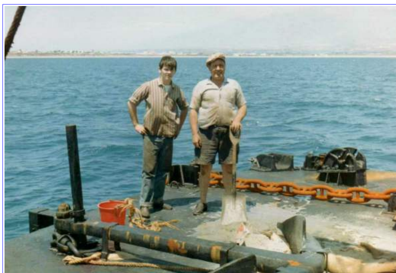
George Hatch and deck boy cement up spurling pipes after pumping out chain lockers on Cinglaise .
