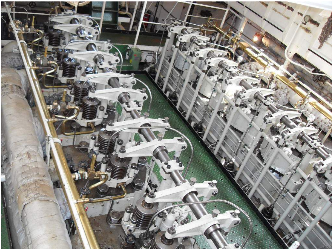
The immaculate engine room of the "Elbe" showing her two 6 cylinder M.A.N. engines
